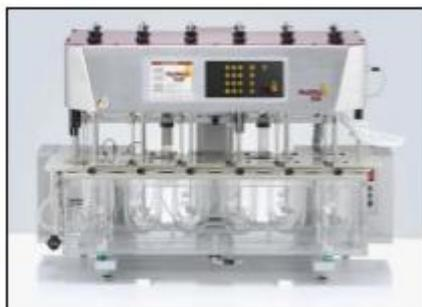
**Figure 27: Appareil de dissolution in vitro**
